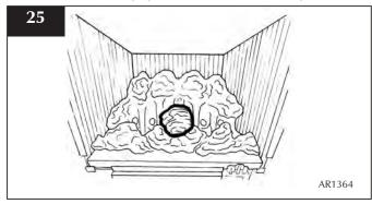
9.8 Place a medium size coal either side of the first large one, in the depressions in the front coal. Resting between the flame baffle and the front coal. See diagram 26.
